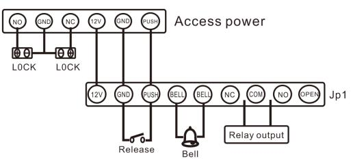
**Remark:** If let relay drive electric-lock, please connect a reverse diode with the lock's "+" and "-" poles.
